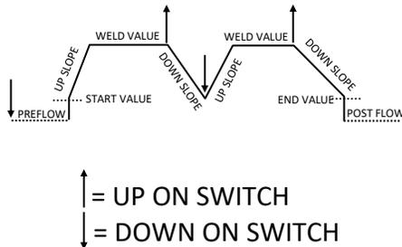
4T Torch Operation Effect on Weld Cycle. (Start/End Values are fixed.)
