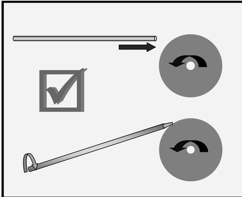
1. Use a dedicated grinding wheel or contamination may result. Do not breath grinding dust! Wear eye protection and gloves.
