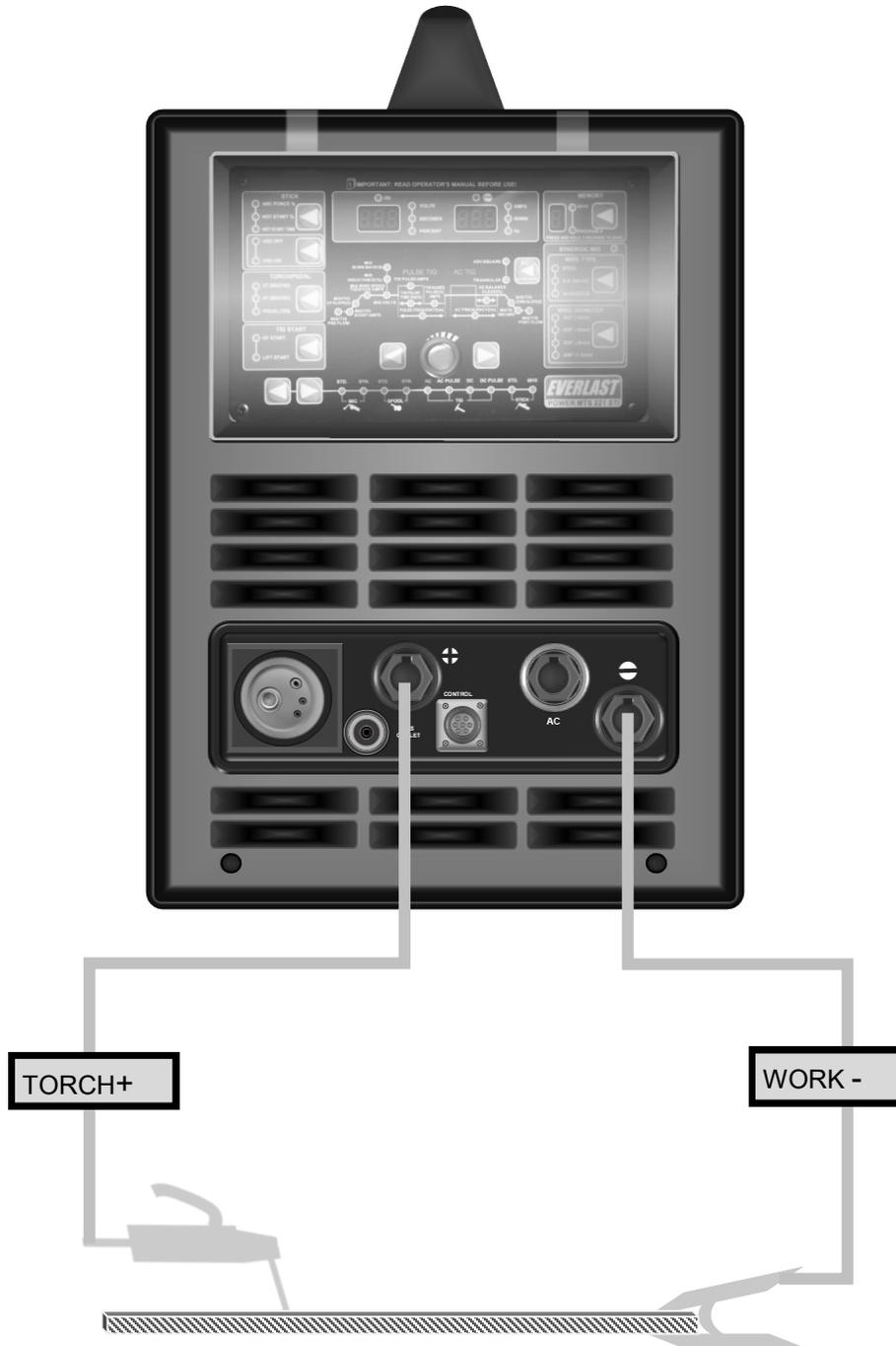
\*This is the typical setup for stick welding. Most all welding electrodes use electrode positive as the preferred polarity. Some will run electrode negative (EN) if needed. Most will not perform well in EN. Consult the electrode manufacturer's recommendations for applications of EN. Usually E6011 is considered to be able to run EN, but runs better EP.
