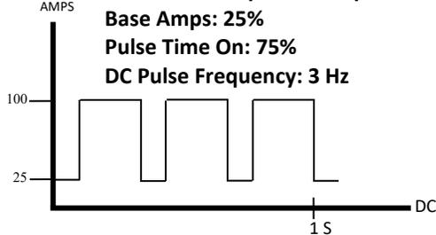
the standard unit “Hertz.” Simply, it is the number of pulses per second that occur. Pulse frequency controls the arc constriction and also helps with heat management.
