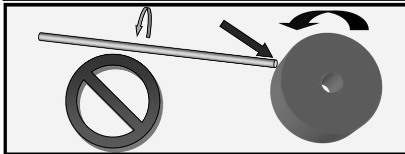
Do not grind the Tungsten parallel to wheel face or an unstable arc will result.
