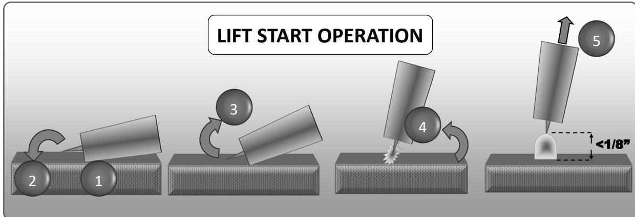
1. Position the edge of the ceramic cup on the metal. Press and hold the torch switch or press the foot pedal. Wait for the Pre-flow to start. (Make sure pre-flow is set for less than .4 seconds or start will be noticeably delayed.)
