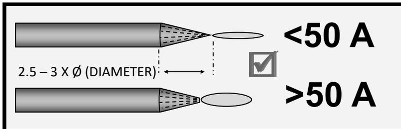
Use a point for low amp use to help control arc. Create a slight truncation on the tip for higher amp use for best arc stability. Grind the tip so that it is 2.5- 3 times longer than the tungsten is wide (Diameter).
