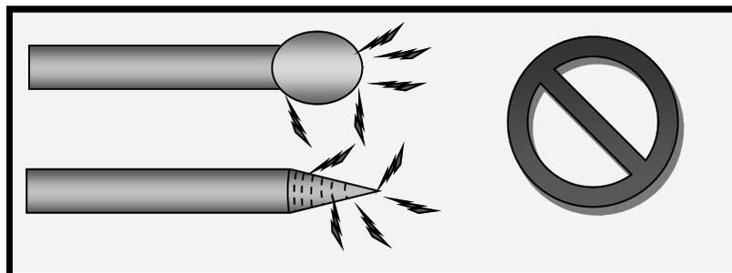
Do not ball the Tungsten while welding, or an erratic arc will result. Make sure that the grinding marks run parallel to the tip. Concentric marks will also cause an erratic arc.
